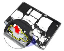
7. Remove the modem connector from the computer.
