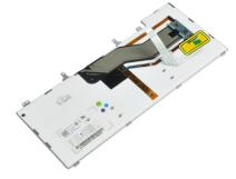
9. Remove the keyboard cable from the keyboard.
