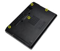
3. Lift the base cover to remove it from the computer.
