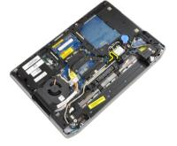
7. Remove the LVDS and camera cable from the routing channel.
