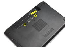
4. Remove the screws that secure the keyboard to the palmrest assembly.
