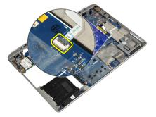
4. Remove the screws that secure the media board to the computer.
