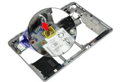
4. Remove the modem cable from the routing channel.
