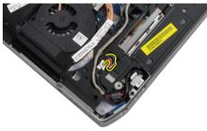
4. Remove the screw that secures the power-connector bracket to the computer.
