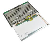
6. Remove the display panel from the display assembly.
