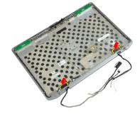
5. Remove the screws that secures the display hinges to the display assembly.
