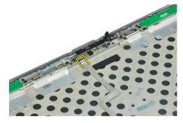
4. Remove the screw that secures the camera to the display assembly.
