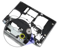
6. Remove the modem-connector bracket from the computer.
