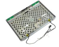
4. Remove the display hinge plates.
