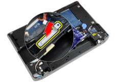
7. Disconnect the LVDS cable from the back of the system board.
