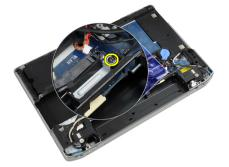
6. Remove the LVDS cable bracket from the computer.
