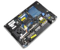
6. Disconnect the camera cable from the computer.
