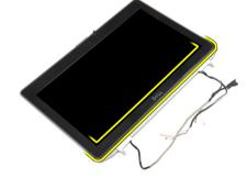
4. Pry up the left, right and top edges of the display bezel.
