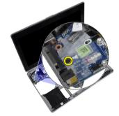
4. Remove the I/O board from the computer.
