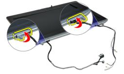
4. Pry loose the edge of hinge cap from the hinge and remove the hinge caps from the display assembly.
