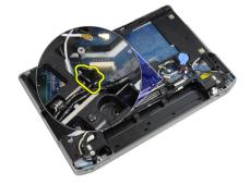
5. Remove the screw securing the LVDS cable bracket.
