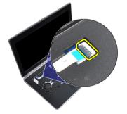
6. Disconnect the touchpad cable from the system board.
