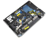
**10.** Remove the screws that secure the display assembly to the computer.
