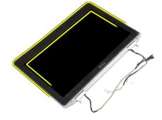
5. Remove the display bezel from the display assembly.
