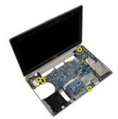
11. Gently lift the left edge of the system board assembly and raise it to a 45–degree angle and release the system board from the port connectors on the right.
