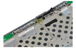
4. Peel back the adhesives securing the LVDS and camera cable to the display assembly.
