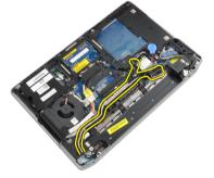
8. Disconnect any antennas connected to wireless solutions.
