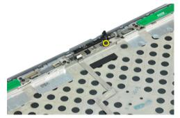
5. Remove the camera from the display assembly.
