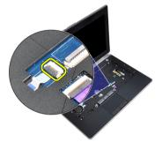
7. Disconnect the SD card cable from the system board.
