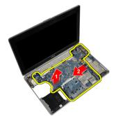
12. Release the system board from the connector port on the back and remove the system board from the system.
