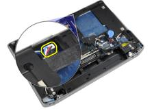
9. Flip the system over and disconnect the media board cable from the system board.
