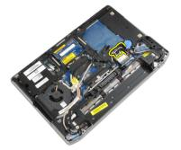
**9.** Remove any antennas from the routing channel.
