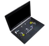
5. Disconnect the LED cable from the system board.
