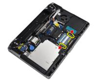
4. Remove the memory module from its connector on the system board.
