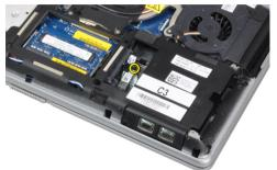
4. Lift up the card along the bottom edge and remove it from the housing.
