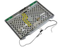
5. Remove the LVDS and camera cable from the display assembly.
