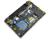
4. Flip the computer over and remove the screws that secure the palmrest assembly to the computer.
