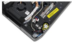
6. Remove the power-connector cable from the computer.
