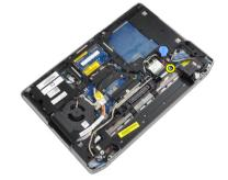
4. Remove the support bracket from the computer.
