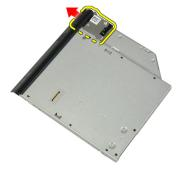
7. Remove the screws that secure the optical-drive latch bracket to the optical-drive assembly
