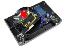
8. Disconnect the speaker cable from the base of the system board.
