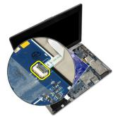
**10.** Remove the screws that secure the system board to the computer.
