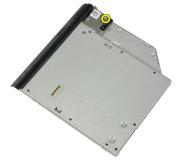
6. Push the optical-drive latch forward and remove it from the optical-drive assembly.
