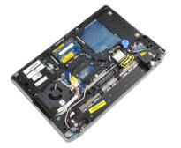
5. Pull upwards on the tab to disconnect the LVDS cable from the computer.
